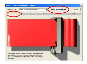
2. Select one of the preset test cuts, then click "Cut Test Now" (make sure the plotter is loaded and initialized first).
